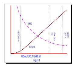
As shown in from the typical performance curves of Figure 1, the high torque at low speed characteristic of the series motor is evident.
