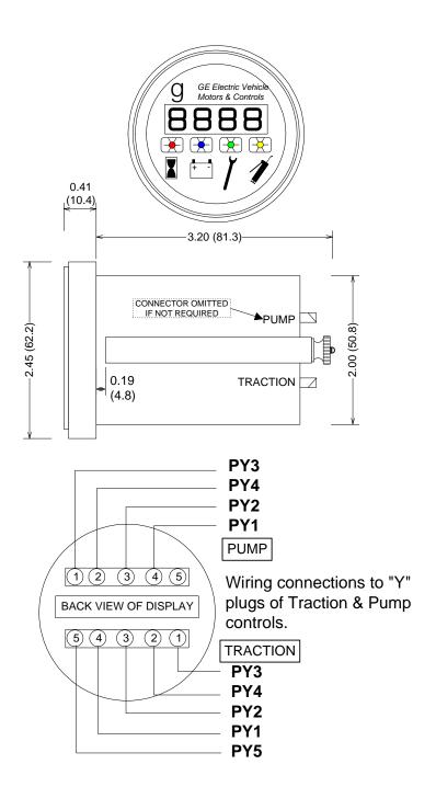
Section 6.6 Suggested Wiring Configuration for Use of GE Standard Traction/Pump Dash Display with Dual Motor Traction System
