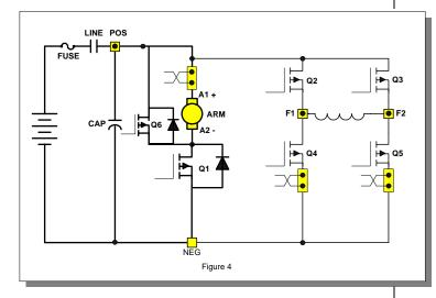
By energizing the transistors in pairs, current can be made to flow in either direction in the field. The field control circuit operates at 2 KHZ, and the armature control circuit typically operates at 12KHZ, a frequency normally above human hearing. This high frequency coupled with the elimination of directional contactors, provides very quiet vehicle operation.
